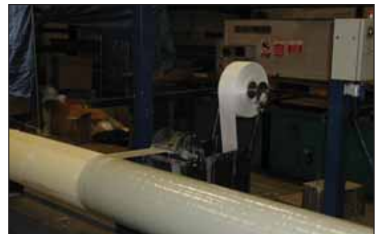
GRP jacketing is applied automatically on pipe segments with high production rate in a controlled environment
